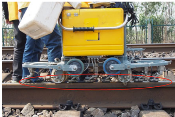
Fig. 2.8 Ultrasonic probe system on the JGT-10 portable rail detector provided by the Lu Chao Ltd (China)
